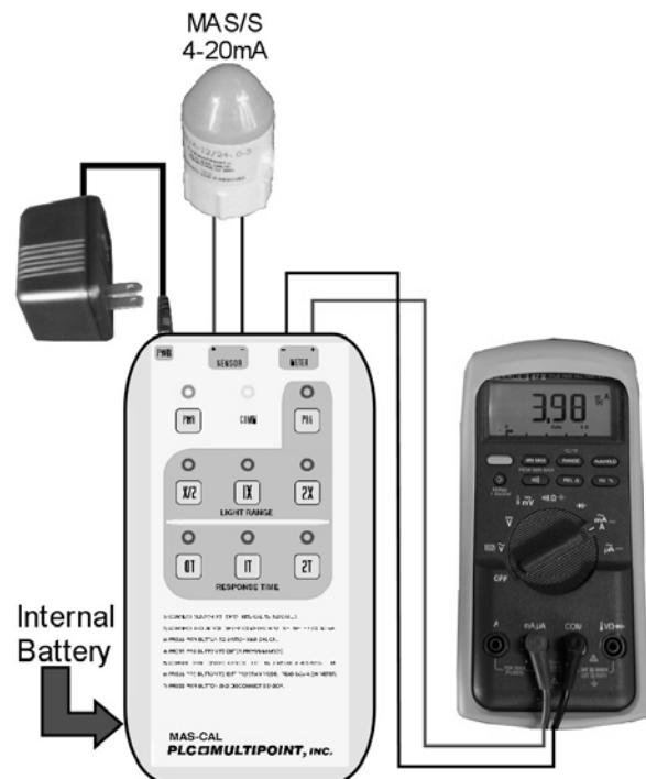
FIGURE 1: MAS-CAL HOOK-UP DIAGRAM
